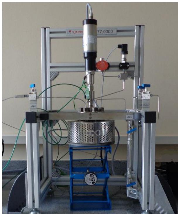
Figure 4. Frame with autoclave
