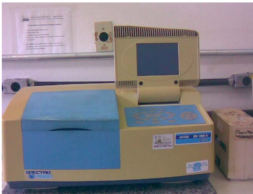
Figura 5.2.2: espectrofotômetro Spectro Vision UV-VIS DB1880S Double Beam
