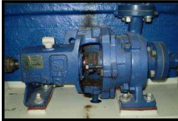
Figura 4.4 – Bomba centrífuga KSB Meganorm 25-150.
