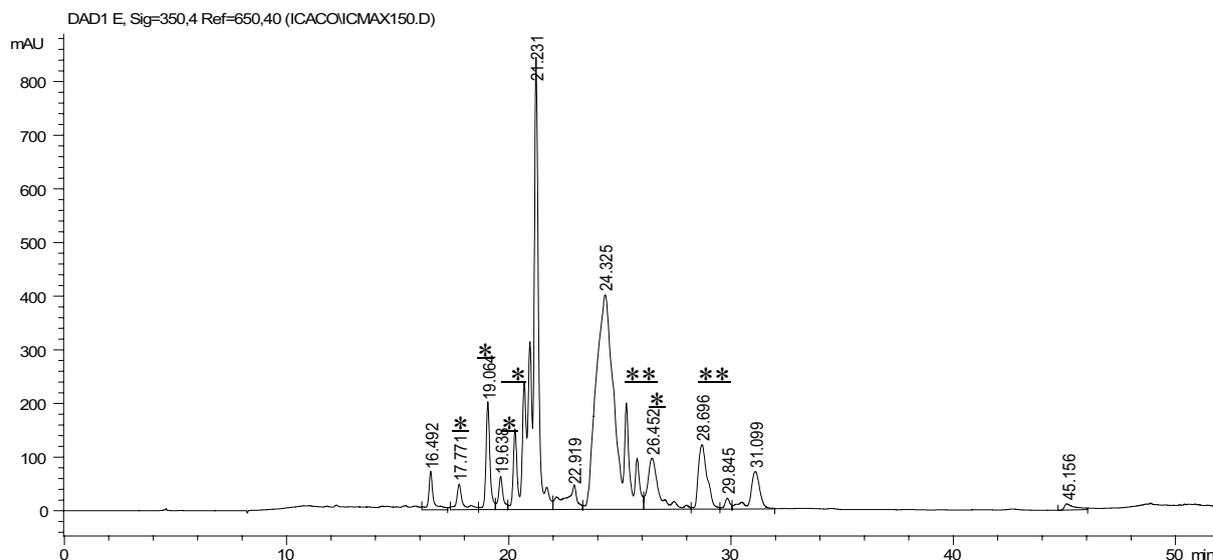
**Figure 2.** HPLC chromatograms acquired at  $\lambda$  350 nm of total hydroalcoholic extract of *Chrysobalanus icaco* L. leaves (column 250 x 4.6 mm Synergy MAX RP-12 (4 $\mu$ ), Phenomenex®, USA). \*Myricetin derivatives, \*\* Quercetin derivatives.
