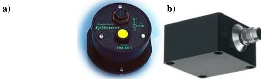
Figura 15 – Acelerômetro “force balance”: a) modelo Kinemetrics FBA ES-T ( http://www.kinemetrics.com ); b) modelo Kistler servoK-Beam ( http://www.kistler.com )
