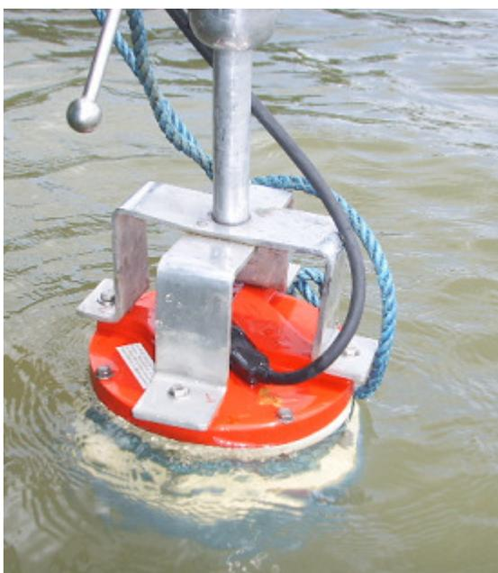
**Figura 4.2** - Acoustic Doppler Current Profiler (ADCP).
