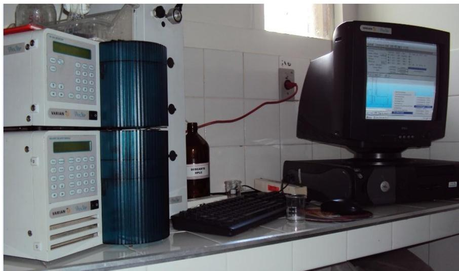
Figura 17- Modelo ProStarVARIAN, com coluna ODS RP18, 25cm X 4mm
