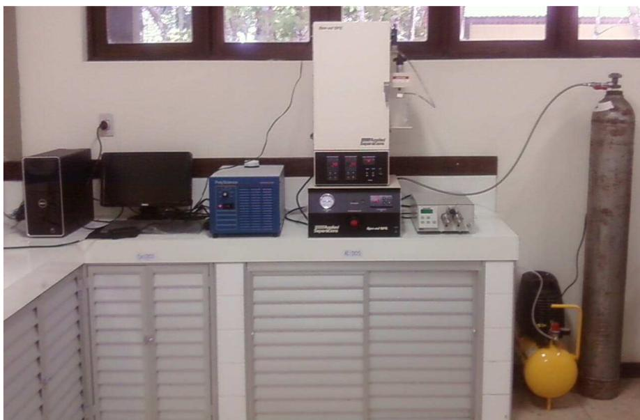
**Figura 3.1** - *Spe-ed<sup>TM</sup> SFE* modelo 7071 da Applied Separations, Inc.
