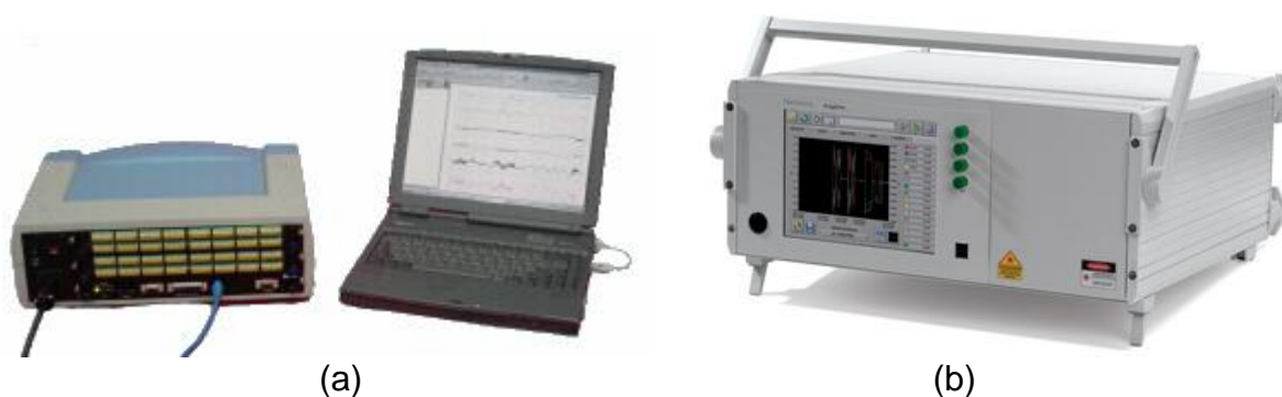
Figura 4.6 - (a) ADS e (b) Braggmeter Benchtop. (Fonte: GSTATIC, 2011 e FIBERSENSING, 2010)
