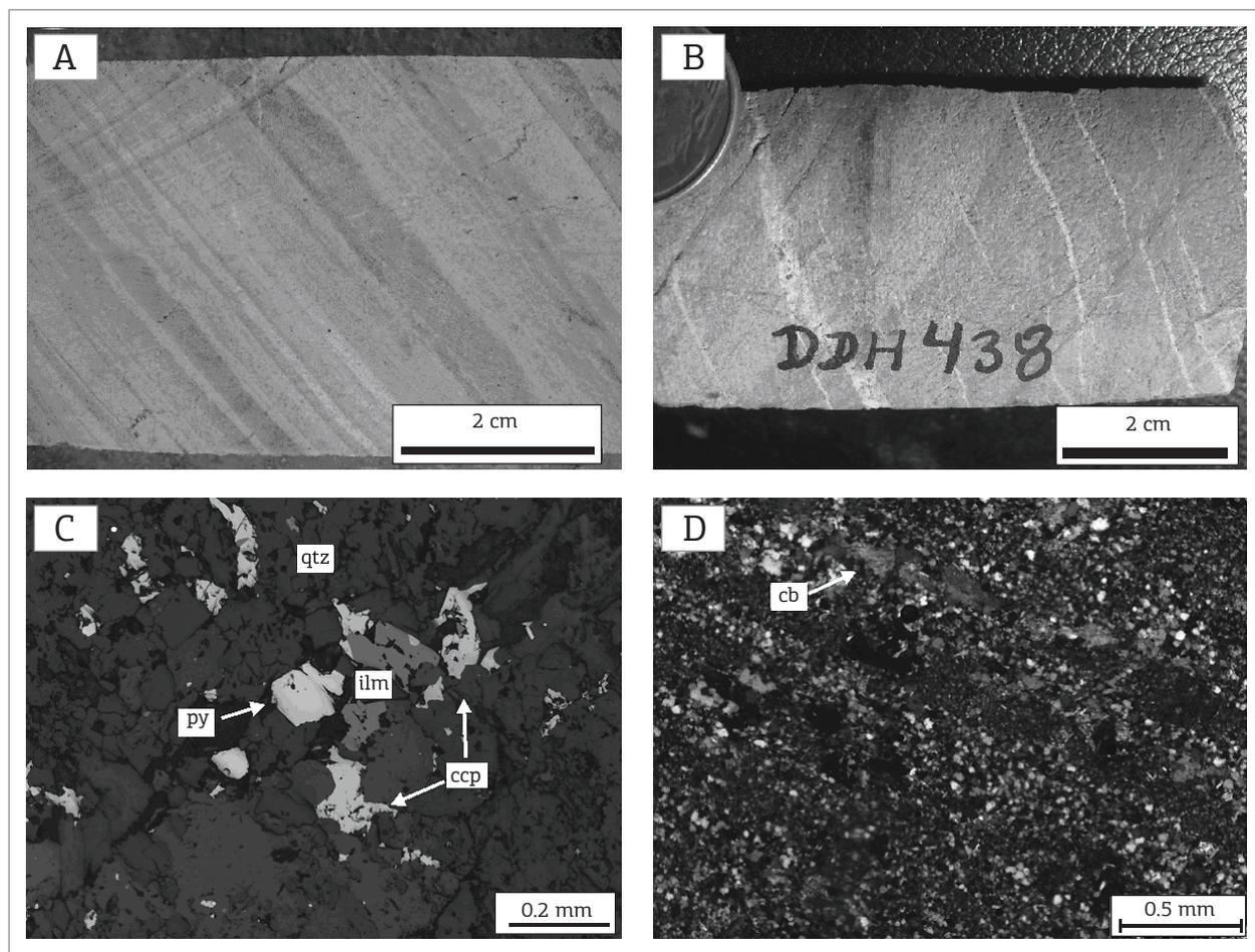
Figure 4. Mesoscopic aspect of the tuffite (A) without hydrothermal alteration and (B) crosscut by carbonate veinlets. At (C) and (D) microscopic detail of sulfide and carbonates, respectively, deposited in fractures between the layers. Mineral abbreviations: ccp: chalcopyrite; ilm: ilmenite; cb: carbonate; qtz: quartz; py: pyrite.
