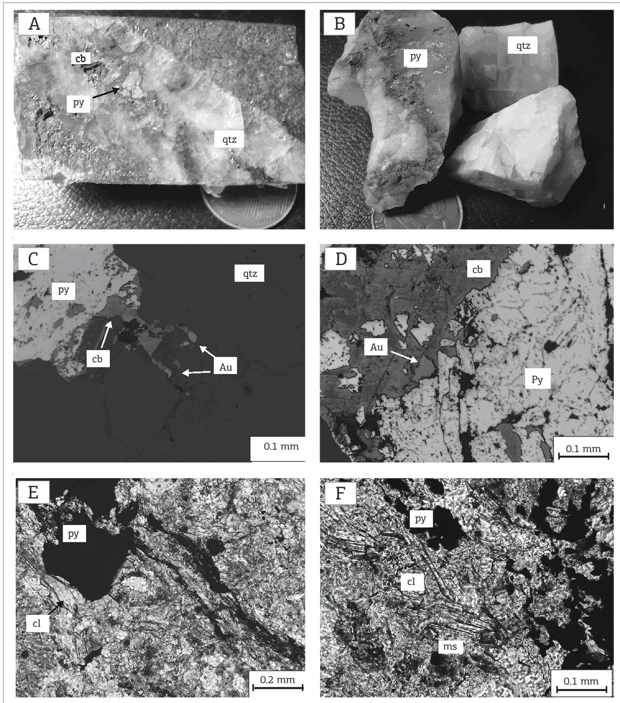
Figure 5. Mesoscopic (A – B) and microscopic (C – F) images showing the form of occurrence of the hydrothermal mineral assemblage at Piaba. Mineral abbreviations: Au: gold; qtz: quartz; py: pyrite; ms: muscovite; cl: chlorite; cb: carbonate.
