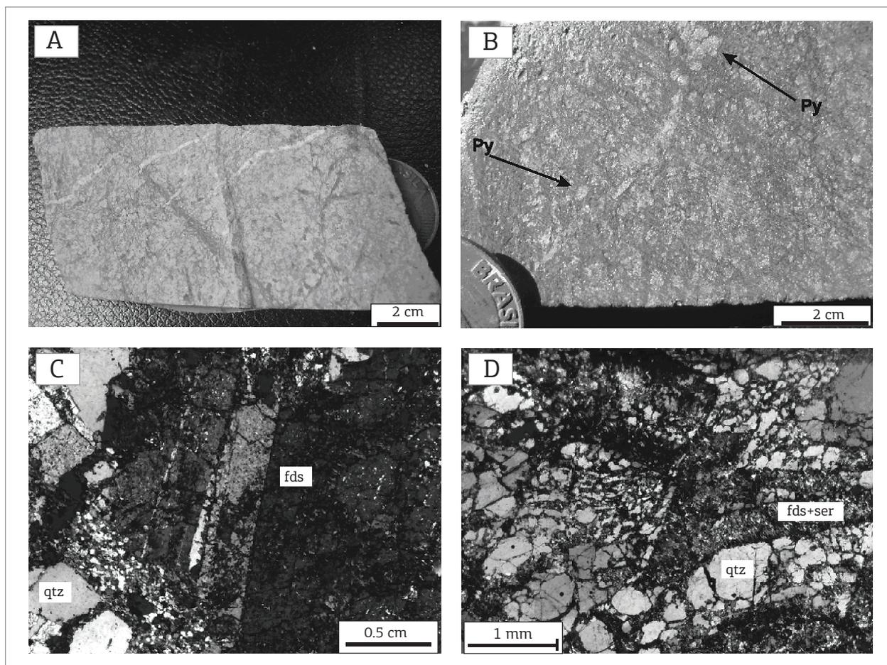
Figure 3. Drill core photographs (A–B) and photomicrographs of the host rocks at Piaba (C–D). Chloritized volcanic rock (A) and fine-grained granophyric granodiorite (B) in the less altered portions of the host rocks, where the feldspar twinnings are still preserved (C), while granophyric texture occurs in portions of brecciated samples (D). Mineral abbreviations: qtz: quartz; fds: feldspar; ser: sericite.
