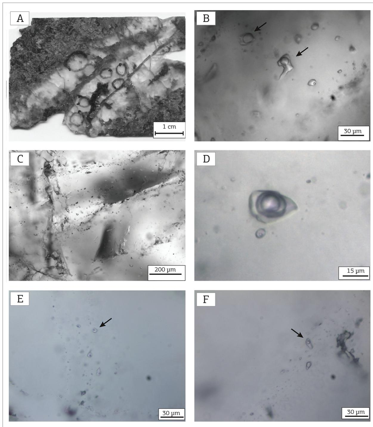
Figure 6. (A) Quartz veinlets with inclusion types (B – F) morphology, size and mode of distribution of the fluid inclusions. Type I (D), Type II (B, E, F) and Type III (C).
