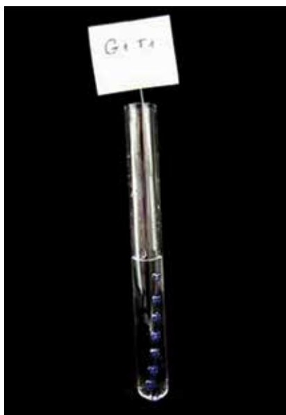
Figure 2 - Specimen in test tube containing artificial saliva.
