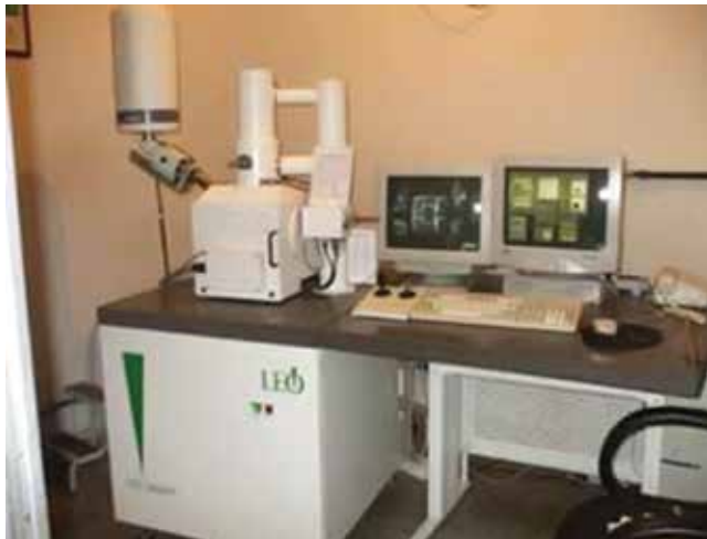
Figure 4 - Leo Zeiss 1450VP Scanning Electron Microscope.
