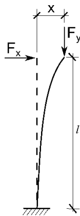
Figura 2.4 – Barra vertical deformada
