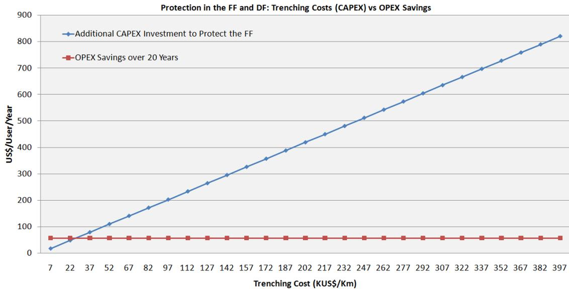
Figure 4.9: Sensitivity analysis showing the protection in the feeder and distribution fiber with trench costs ranging from 7000US\$/Km to 67.000US\$/Km.
