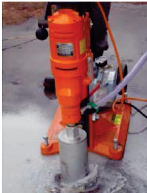
**Figure 14 – Testimony's length standardization and end surface regularization**
