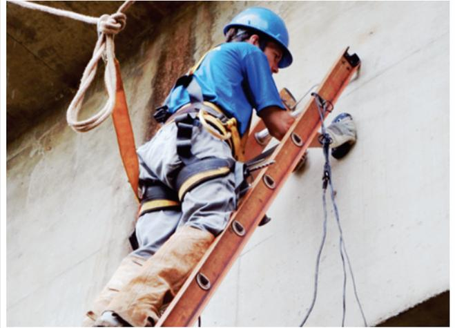
Figure 9 – Pacometry testing on caisson T7
