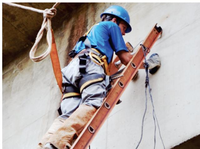
Figure 9 – Pacometry testing on caisson T7
