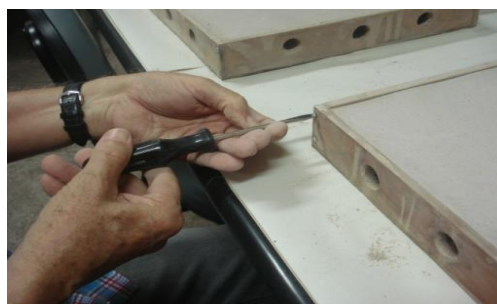
Figura 3.46: Desparafusando as formas.Foto: Amanda Farias (2014).
