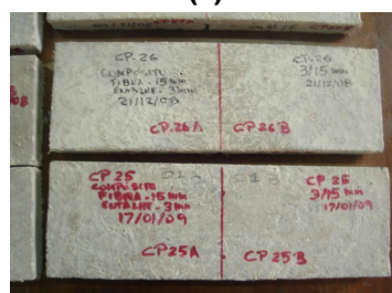
Compósito com entalhe 3,0 mm, comprimento da fibra 15,0 mm
