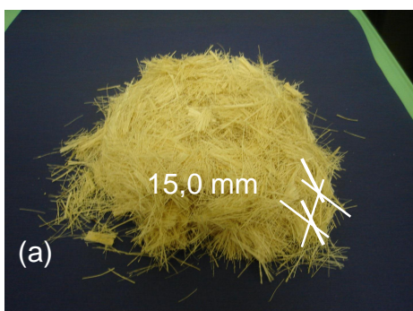
Figura 10 (a) - Fibra de sisal com 15,0 mm de comprimento
