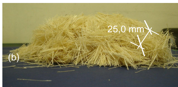
Figura 10 (b) - Fibra de sisal com 25,0 mm
