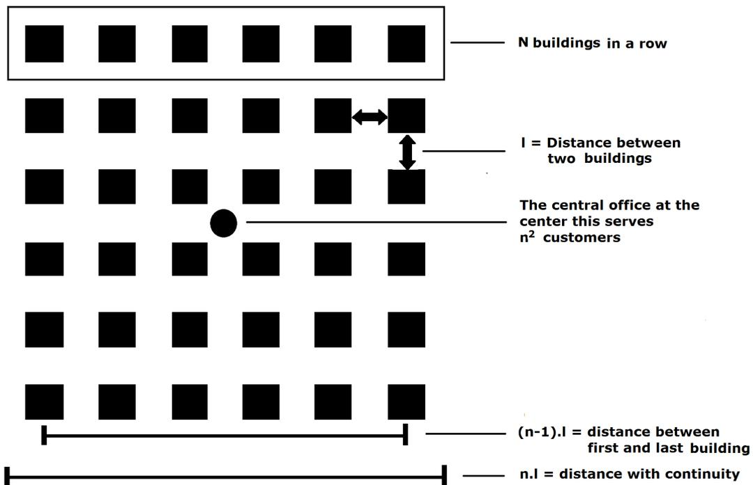
Figure 3.8: Schematic overview of the logical structure and parameters to obtain the trenching and installation distances.
