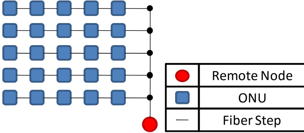
Figure 4.3: Representation of fiber feeding in the quadrant of a certain block.
