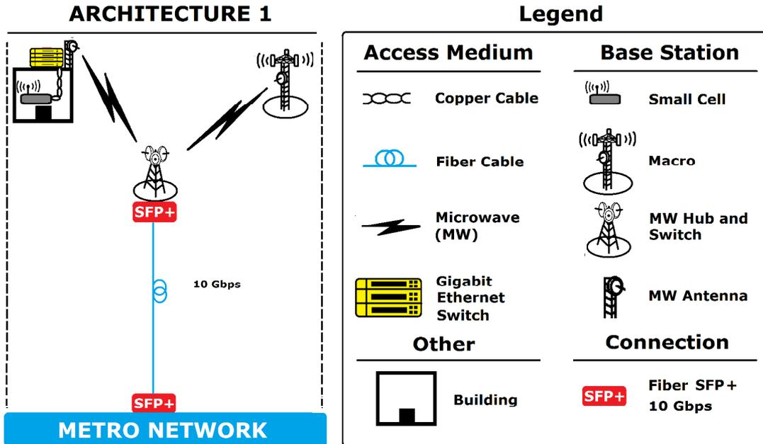
Figure 3.2: Microwave to femto and macro base stations.
