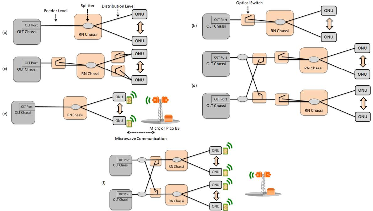
Figure 4.5: Topologies for schemes under investigation. (a) PON with no protection scheme. (b) PON with protection in the feeder fiber. (c) PON with protection in the feeder and distribution fiber. (d) PON with protection in the OLT and feeder fiber. (e) PON with protection using microwave. (f) PON with protection in the OLT and using microwave.
