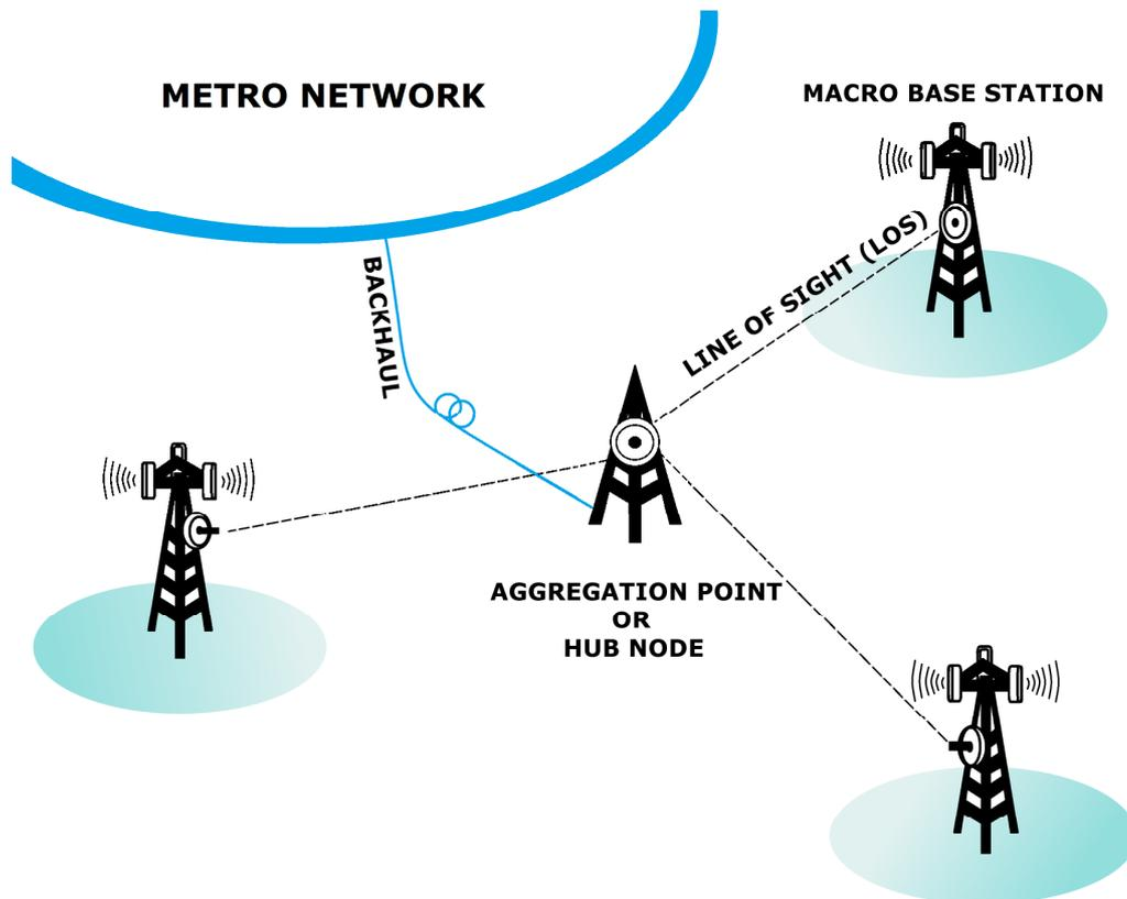
Figure 2.4: Point-to-multipoint microwave backhaul communication.
