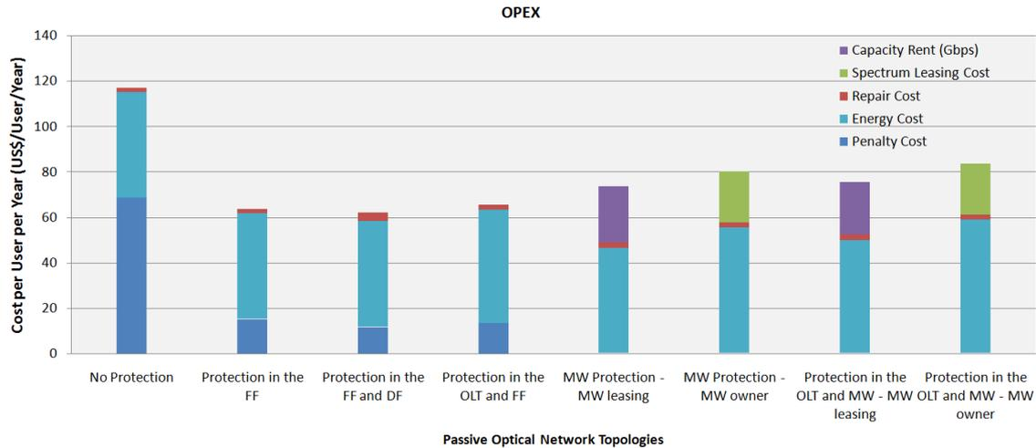
Figure 4.7: A comparison of expenditure in operational undertakings within different PON topologies.
