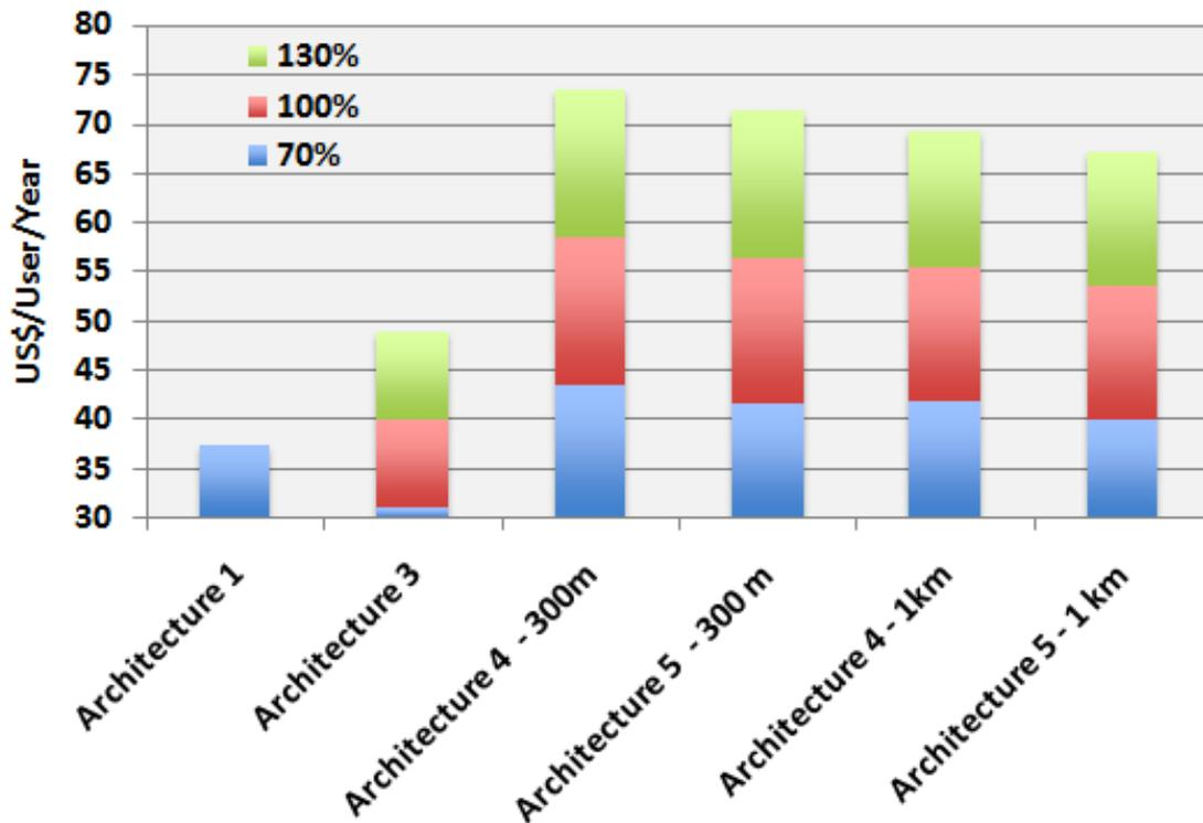
Figure 3.14: Sensitivity analysis of variations in the trenching cost in a range of 70% to 130% of the market price.
