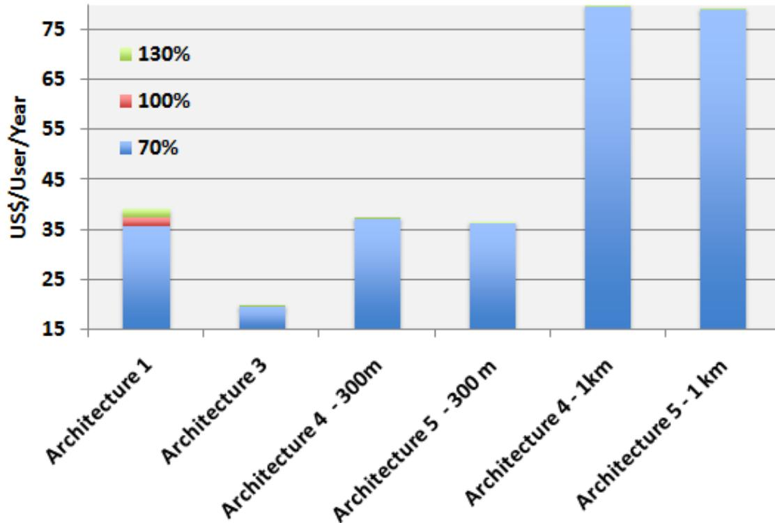
Figure 3.17: Sensitivity analysis of the MW spectrum cost when it varies from 70% to 130% of the market price.
