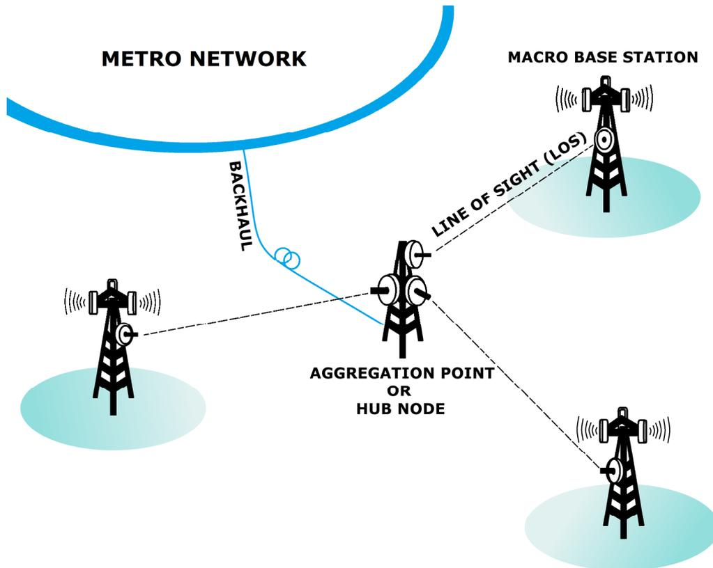
Figure 2.3: Point-to-point microwave backhaul communication.
