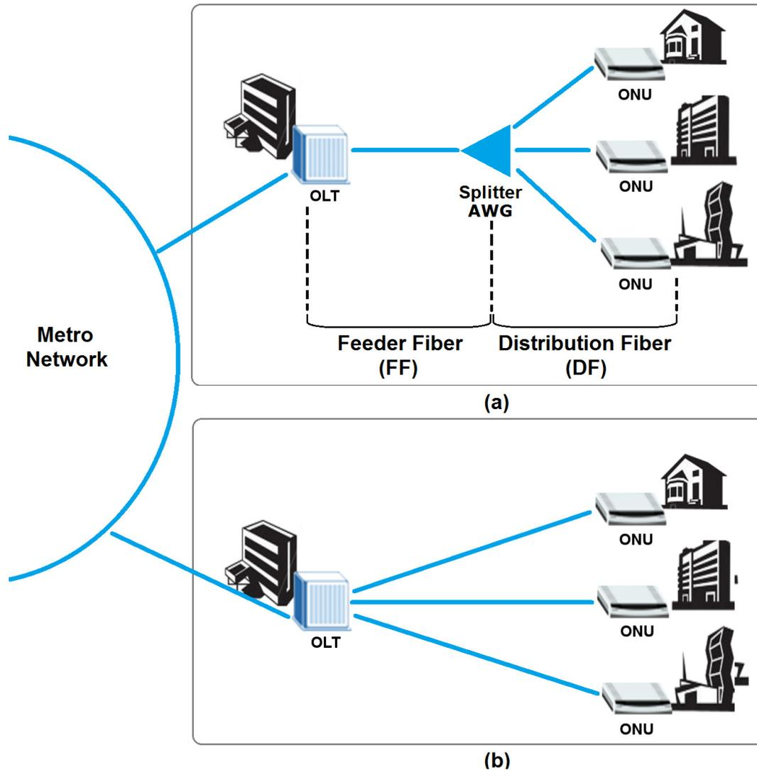
Figure 2.2: Fiber-to-the-home backhaul infrastructures. (a) Passive optical network. (b) Point-to-point fiber architecture.
