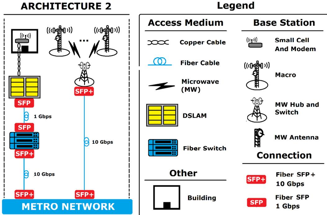
Figure 3.3: Fiber-to-the-node for the femto and microwave to the macro.
