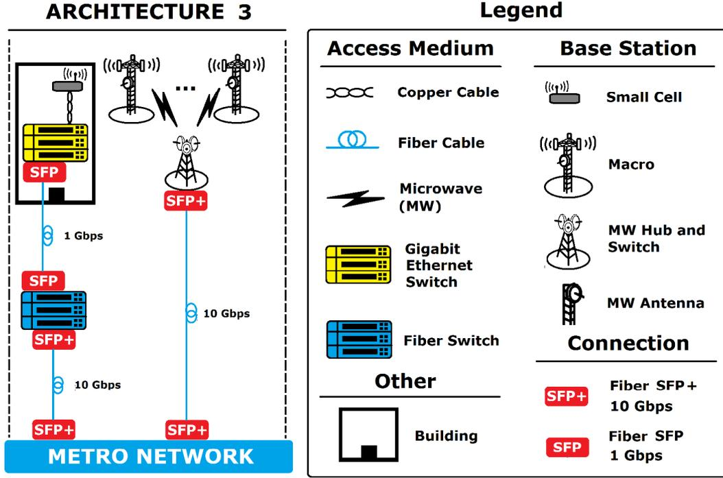
Figure 3.4: Fiber-to-the-building for the femto and microwave to the macro.
