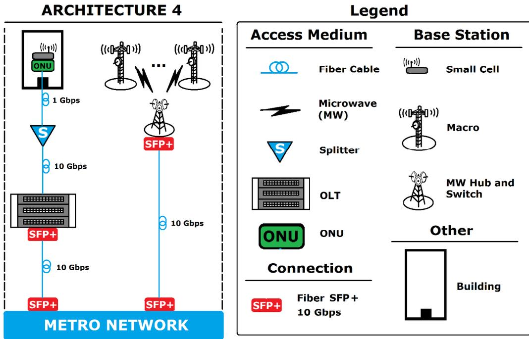
Figure 3.5: Fiber-to-the-home for the femto and microwave to the macro.
