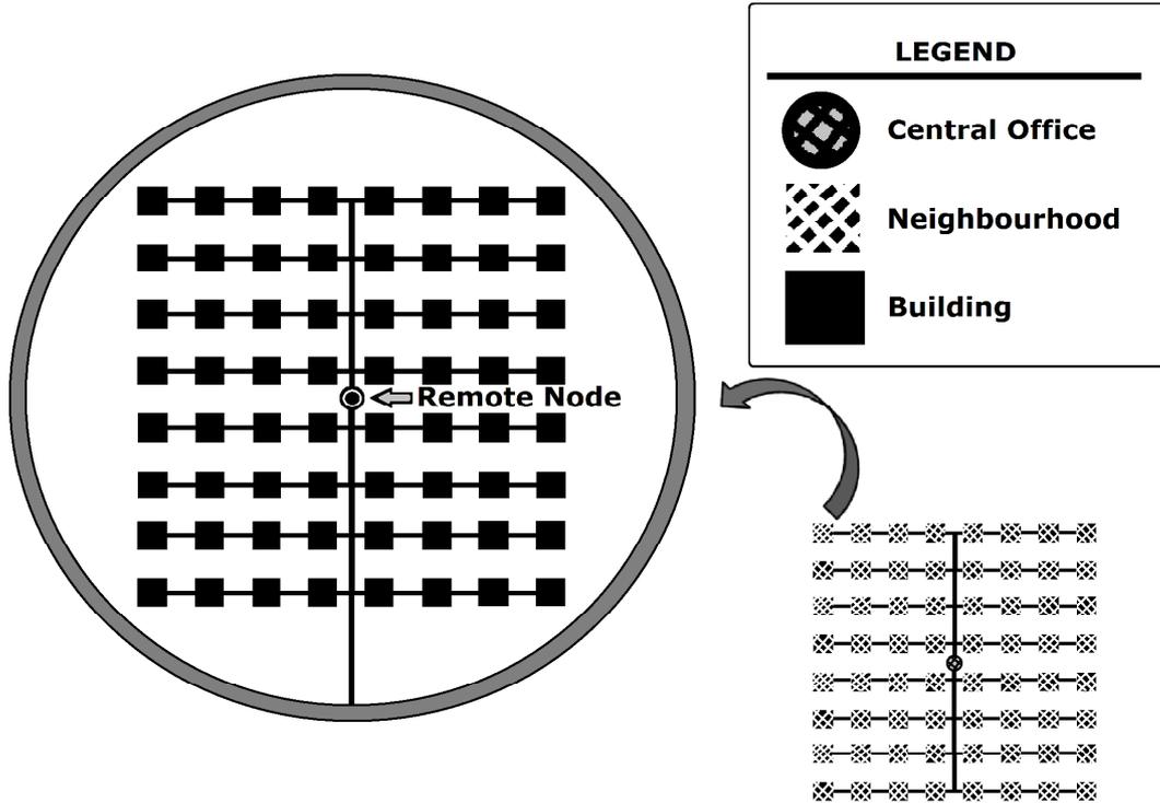
Figure 4.1: Schematic overview of the logical structure of a city with passive optical networks.
