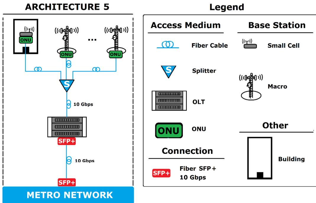
Figure 3.6: Fiber-to-the-home for the femto and macro base stations.
