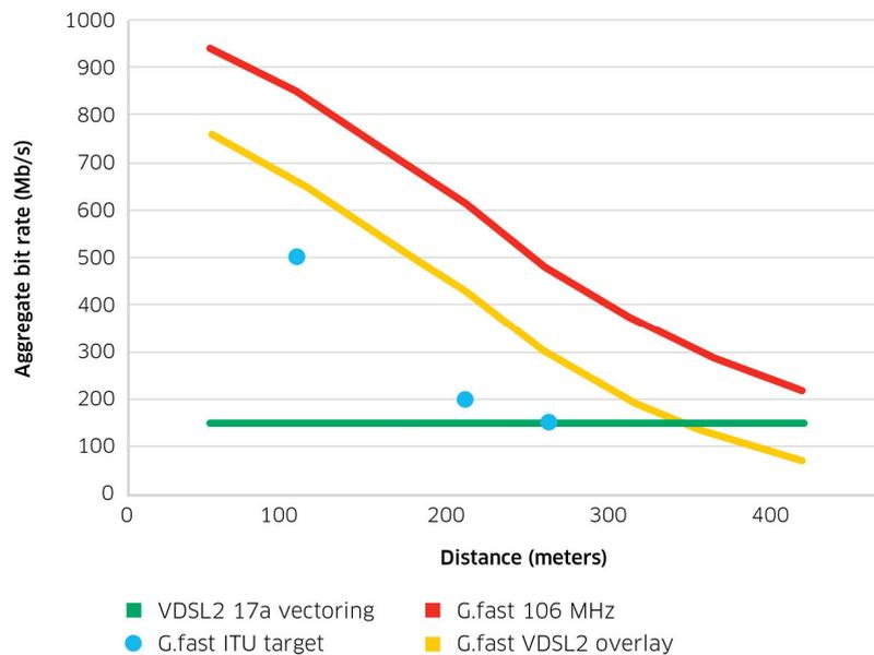
Figure 2.6: Beyond VDSL2: G.fast delivers fiber speeds over short copper loops [65].
