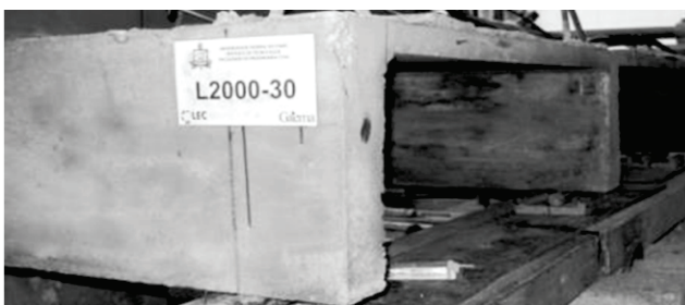
Figura 10 – Groups L1300 e L2000 of slabs with different tables' thickness
