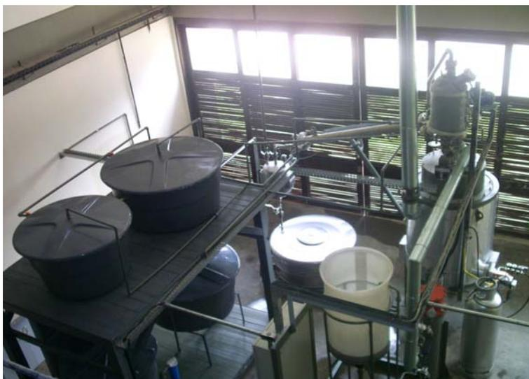
**Figure 3. 1** - View of Thermal Catalytic Cracking Pilot Plant.
