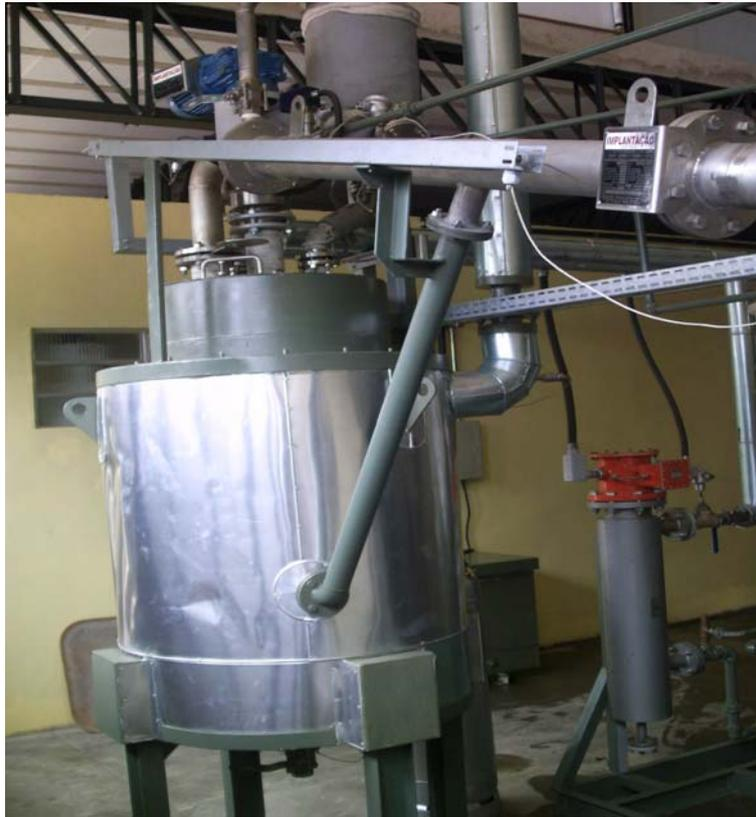
**Figure 3. 2** - Stirred Sludge Bed Reactor (R-01).
