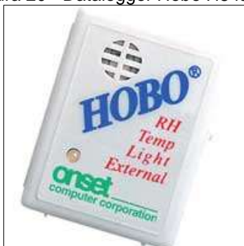
Figura 20 - Datalogger Hobo H8 family
