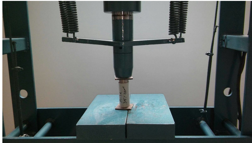
Figure 3.1 – Picture of the hydraulic press that is used to simulate de overburden effect in the samples.
