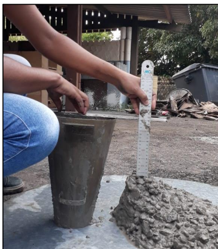
Figura 3.34 – Slump test do concreto
