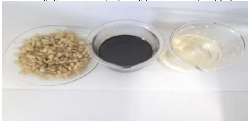
Figure 2: Cross-linked PMMA-based dental resins scraps, liquid reaction products (Dark Liquid) obtained after pyrolysis at 345, 405, and 420°C, 1.0 atmosphere, in pilot scale, and MMA (Colorless Liquid) obtained by fractional distillation of liquid reaction products.
