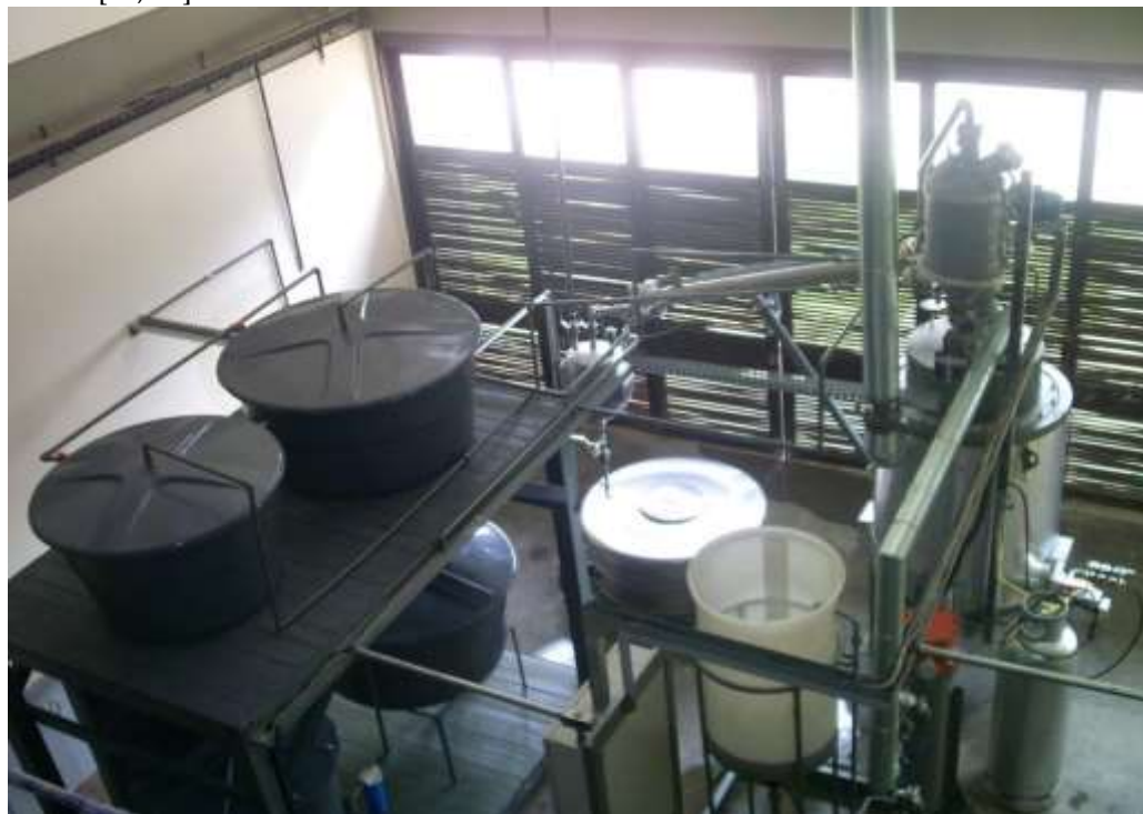
Figure 3: Experimental apparatus (Thermal Catalytic Cracking Unit) for the pyrolysis of cross-linked PMMA-based dental resins scraps at 345, 405, and 420°C, 1.0 atmosphere, in pilot scale.
