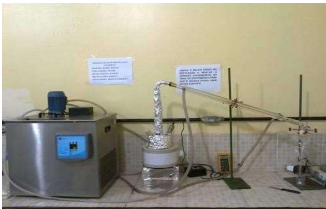
Figure 4: Vigreux borosilicate-glass distillation column of 500 ml, connecting column, condenser, and separator funnel.
