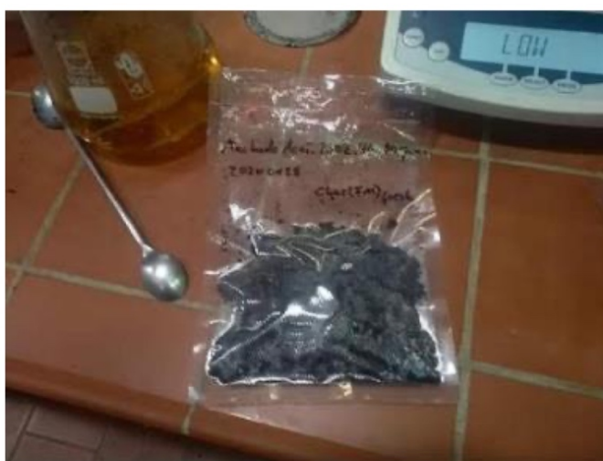
Figure 3. Solid phase (bio-char) and aqueous phase (orange) reaction products.
