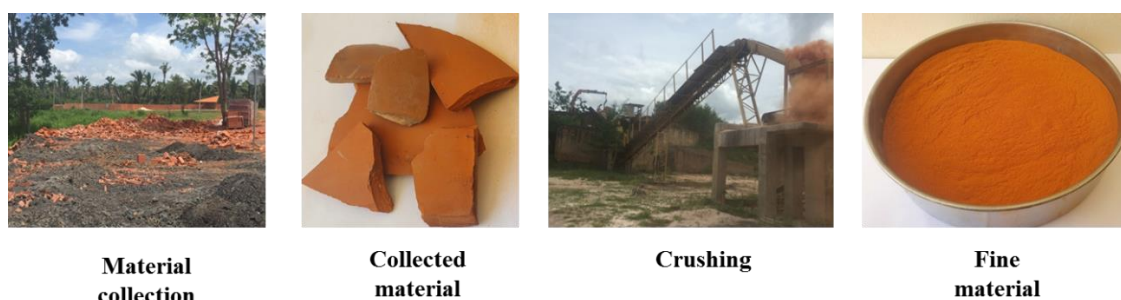
Figure 2. Red ceramic acquisition process
