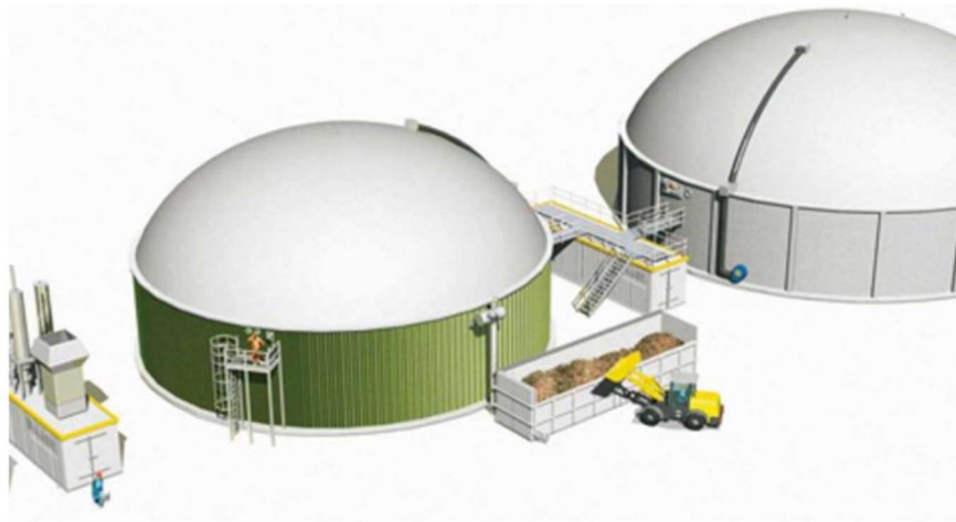
Figura 11 - Biodigestor (Planta Industrial)
