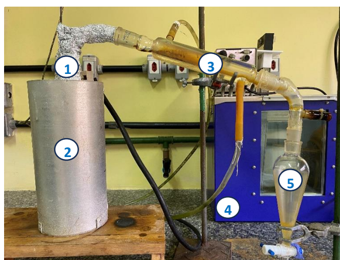
Figure 3. Experimental setup of the pyrolysis process.
