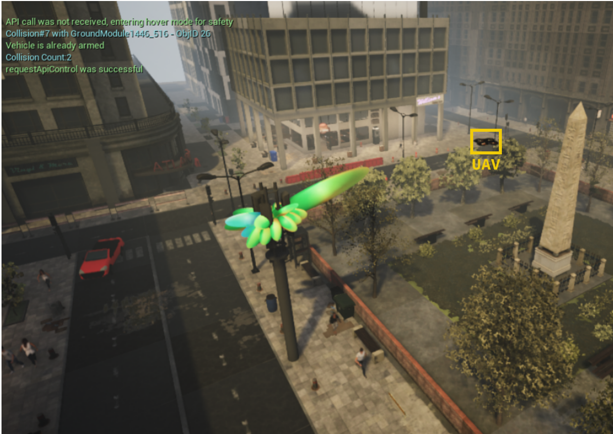
Figure 1.1: CAVIAR simulation scenario, depicting the radiation pattern (in light green) corresponding to the chosen beamforming codebook index to serve a drone (at the right).
