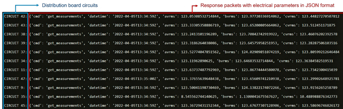
Figure 16. Logs of receiving parameters from the switchboard circuits.
