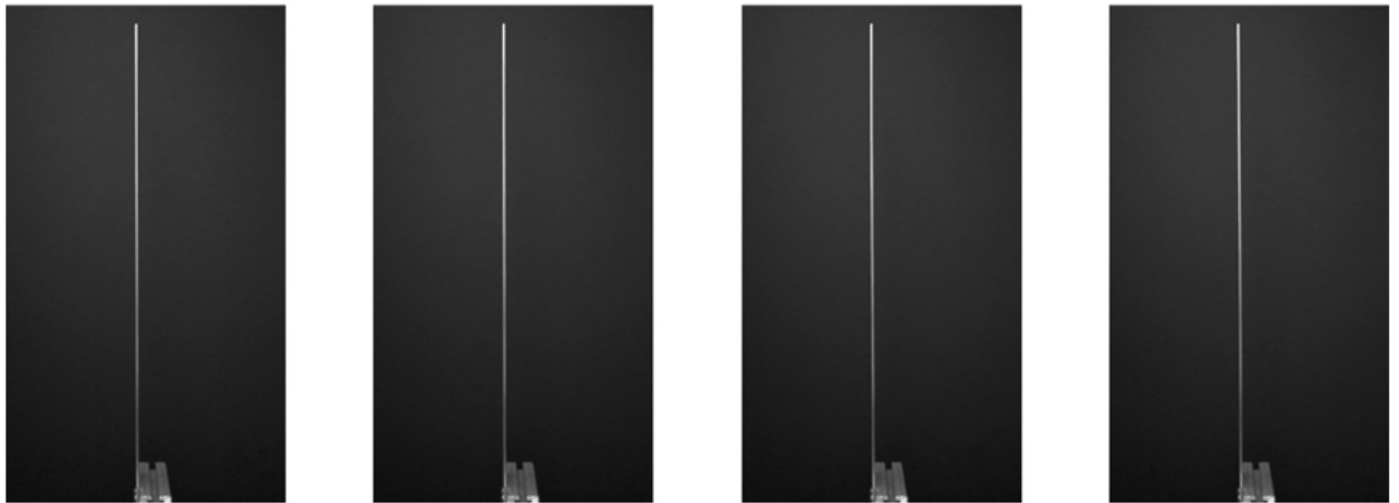
Figure 8 – A few temporal frames from the video measurement of the cantilever beam structure subjected to horizontal excitations.
