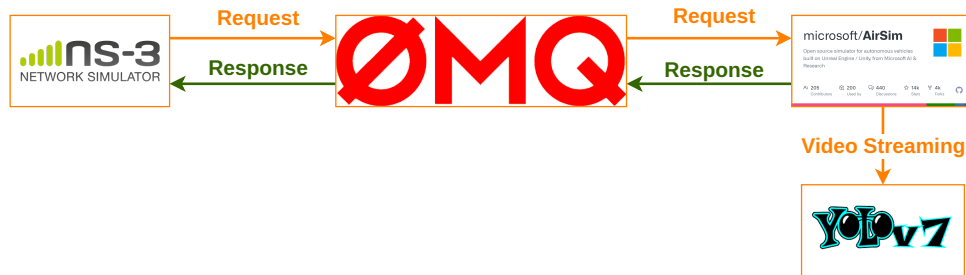
Figure 3.6: Illustration of the messages exchanged between the CAVIAR modules
