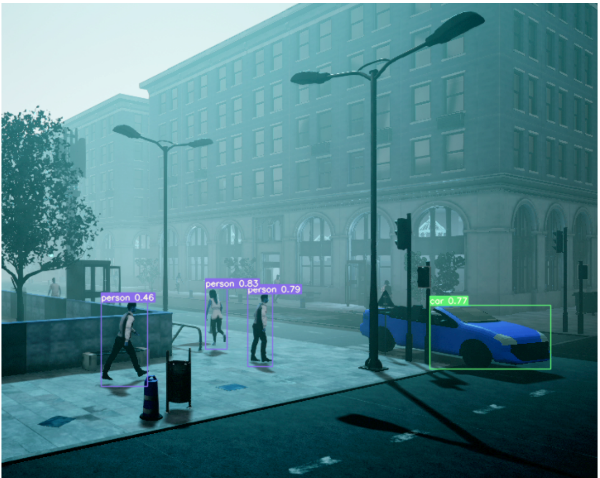
Figure 4.5: Object detection result generated by the AI module
