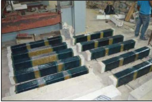
a) Hasnat *et al.* (2016)
