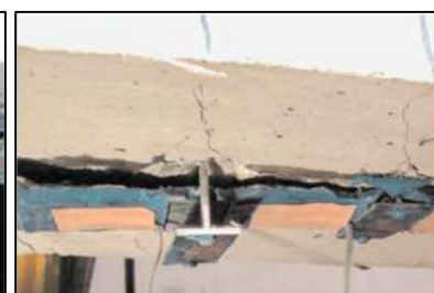
c) Arrancamento do HBF-RP (S4)
