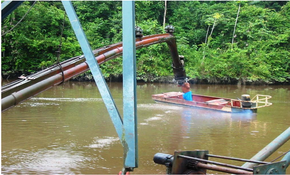
Figure 27: Draga extracting the alluvial deposits, Mazaruni River
