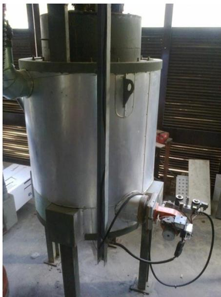
**Figura 13:** Reator de craqueamento (R01)
