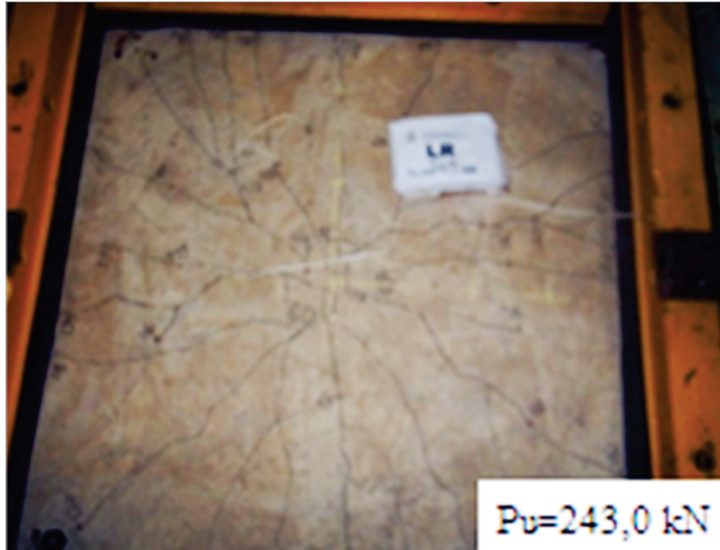
Figure 9 - Cracking pattern of tested slabs
