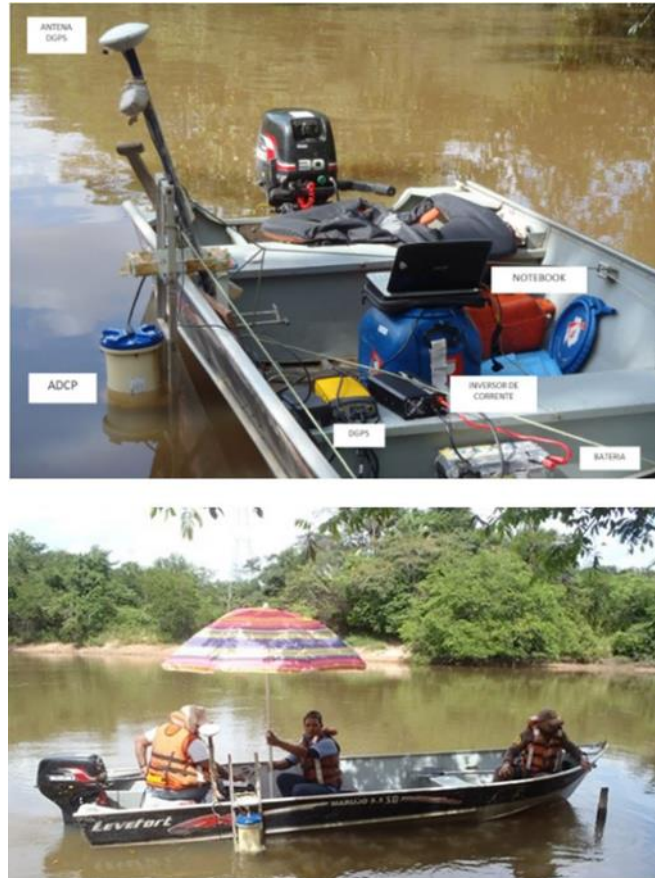
Figure 5. Equipment and vessels used in flow measurements in the rivers within the Itacaiúnas River basin.
