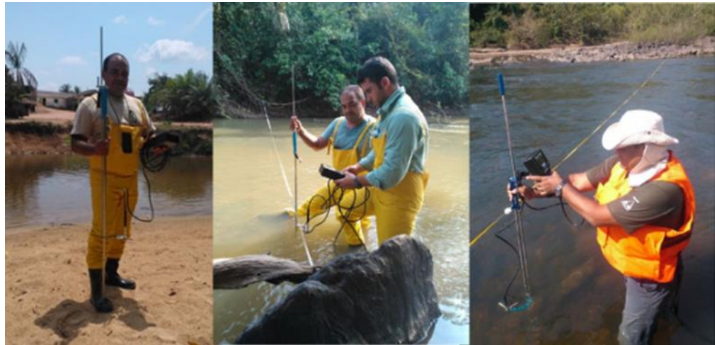
Figure 6. Photos of flow measurement with FlowTracker.
