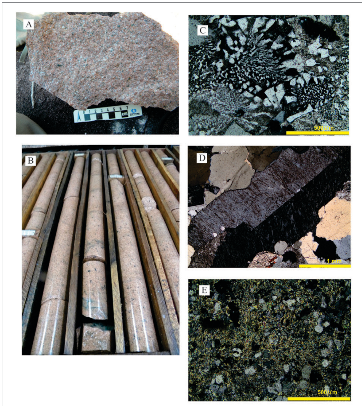
FIGURE 10 – Aspects of the Serra Alkali Feldspar Granite. A) Fine-grained equigranular pinkish granite; B) drill holes from the Coringa deposit with the same granite of “A”; C) granophyric texture; D) twinned potassium feldspar crystal; E) sericitization of potassium feldspar.
