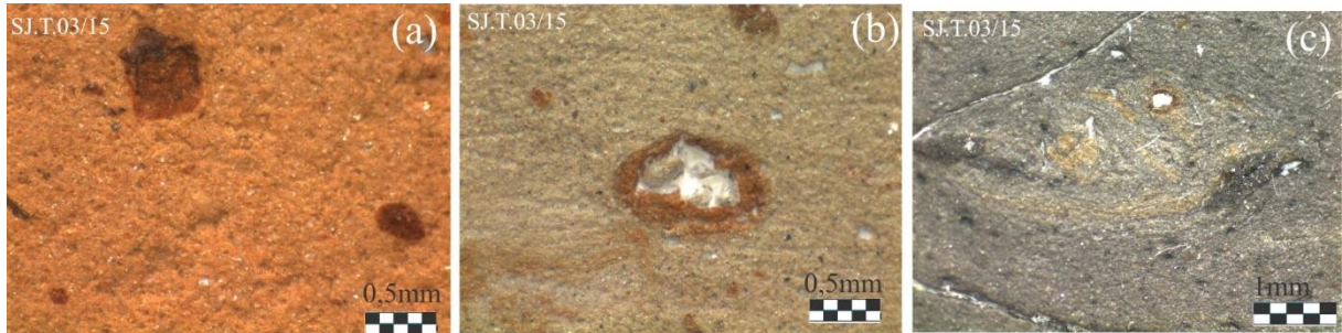
Fig. 24. Photomicrographs of a polished section of RCBC from FSJM (SJ.T.03/15 sample) where non-homogeneous fired is observed: (a) external surface of orange color in sandy silica mass with nodules of Fe-oxyhydroxide and meager quartz grains; (b) intermediate area of light gray color with white nodule aureolated of brown possibly hematite stain; (c) gray central nucleus and white nodules or halos in brown and ochre.
