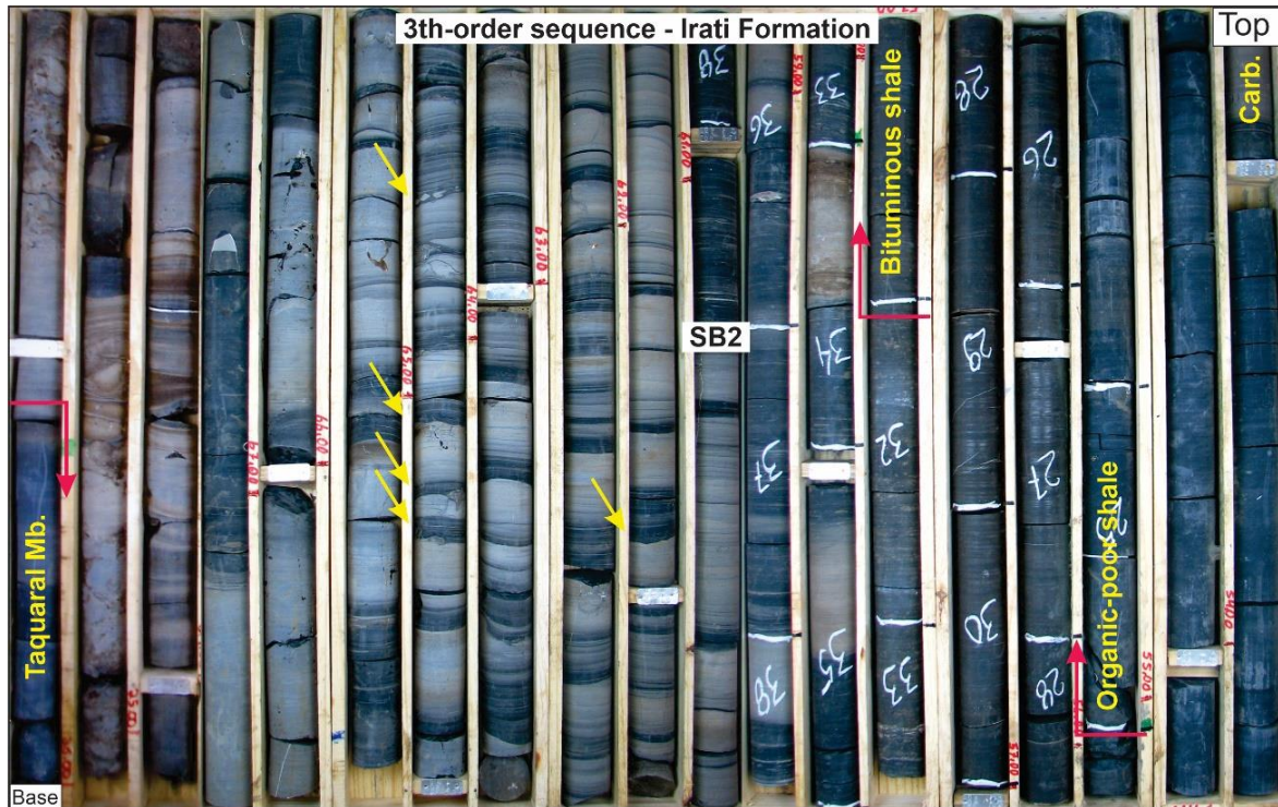
Fig. 5. Core photographs of the second 3rd-order sequence of the mixed deposits (S2). The sequence is overlying the breccia facies in the base of Assistência Member. Note the high-frequency cycles with shallowing-up patterns and the predominance of deepening upward trend of the sequence.
