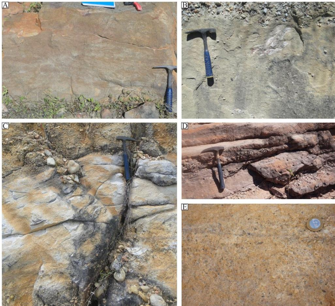
Figure V.7- Massive sandstone lithofacies aspects. A to D) Varieties of massive sandstone thickness beds observed in outcrops interbedded with massive conglomerate horizons. E) Detail of massive sandstone lithofacies clasts morphologies. The hammer length is 30 cm.
