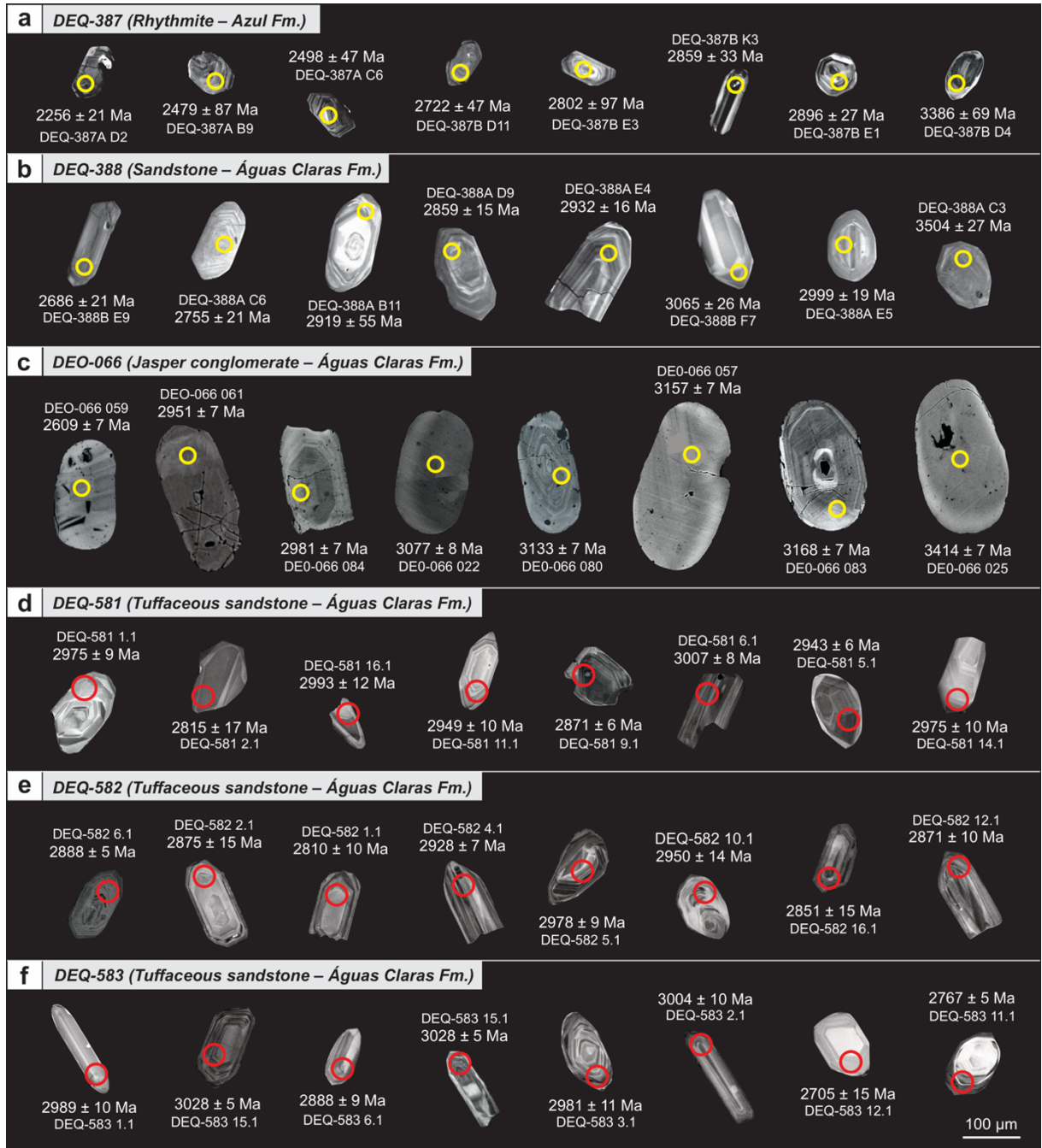
Figure 7.8: Cathodoluminescence (CL) images of some zircon grains dated (U-Pb) with their respective values of ^{207}\text{Pb}/^{206}\text{Pb} dates. (a) Zircon grains dated from the Azul Formation. (b–f) Zircon grains dated from the Águas Claras Formation. The yellow and red circles indicate the site of the laser spots positioned for dating using LA-ICPMS and SHRIMP, respectively.
