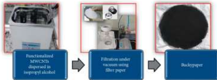
FIGURE 2: Manufacturing process of the BP by vacuum filtration.
