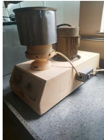
Figure 2. Knife mill utilized for grinding WEEE plastic to adequate particle size to be fed into the pyrolyzer.
