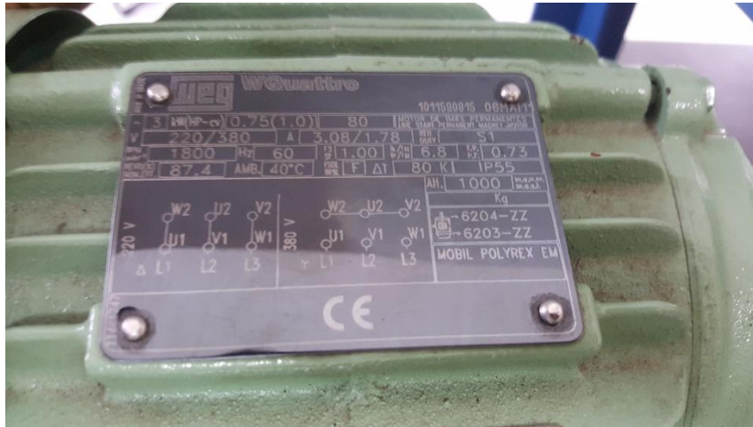
Figure 0-5 – IE4 Class line-start permanent magnet motor nameplate.
