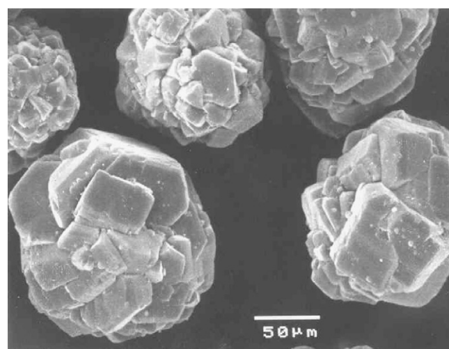
Fig. 4. Electron scanning microscopy of \gamma -alumina produced at 773 K.
