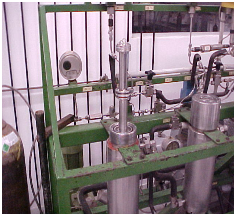
Photography 2: Assemble used to measure the solubility by the dynamic method.
